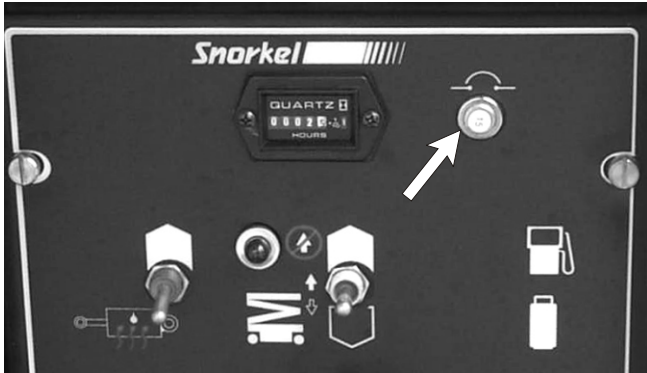
Figure 5.4 - Main Circuit Breaker
