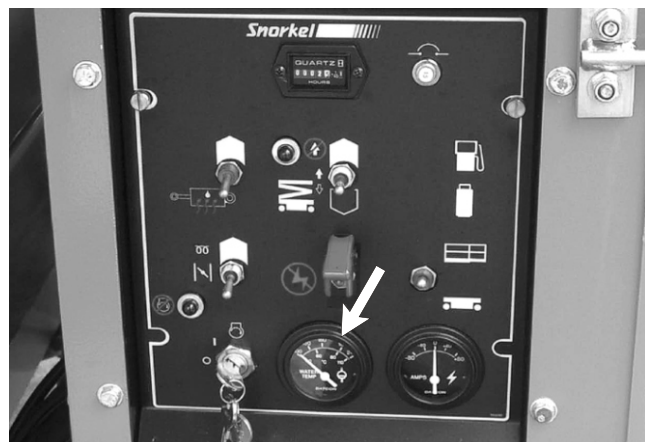
Figure 4.1 - Water Temperature Gauge
