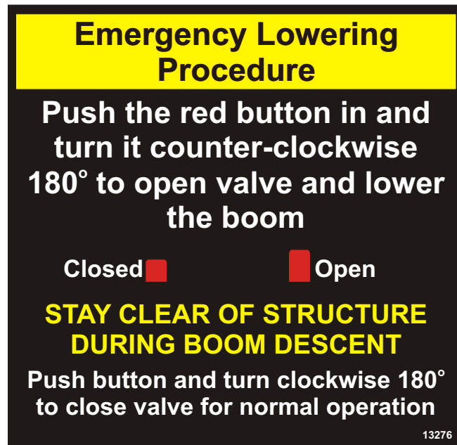
Figure 9.7 - Manual Lowering Procedure Decal
