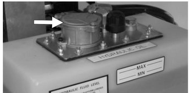
**Figure 7.10 - Hydraulic Oil Filler Cap**
