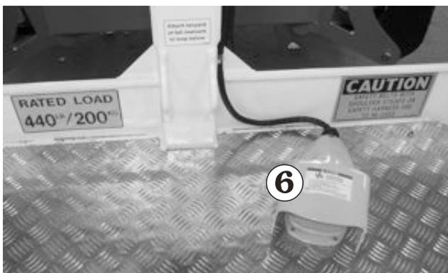
**Figure 8.11 - Platform Foot Switch**
