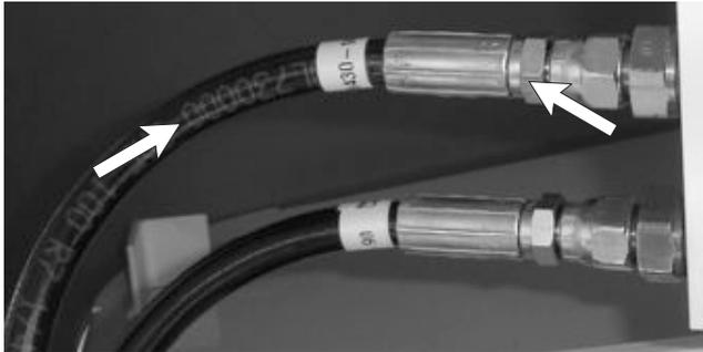
**Figure 7.12 - Hydraulic Oil Leaks At Fittings And Hoses**
