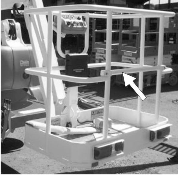
**Figure 2.4 - Gravity Gate**
