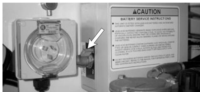
**Figure 11.2 - Master Battery Isolate Switch**
