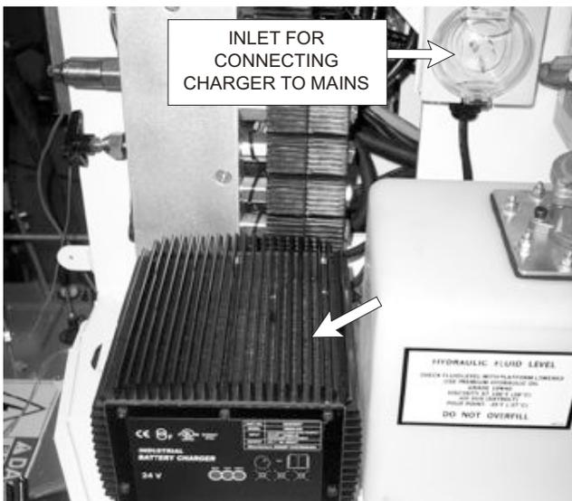
Figure 11.6 - On-Board Battery Charger
