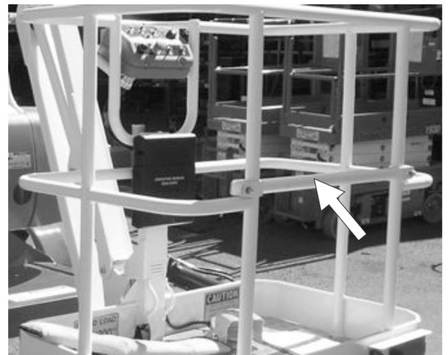
**Figure 7.19 - Platform Gravity Gate**
