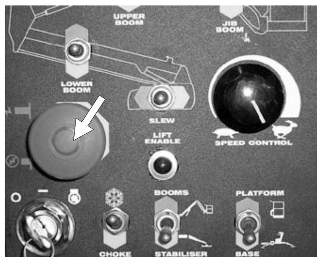
Figure 8.1 - Ground Control Box Emergency Stop Switch Location.
