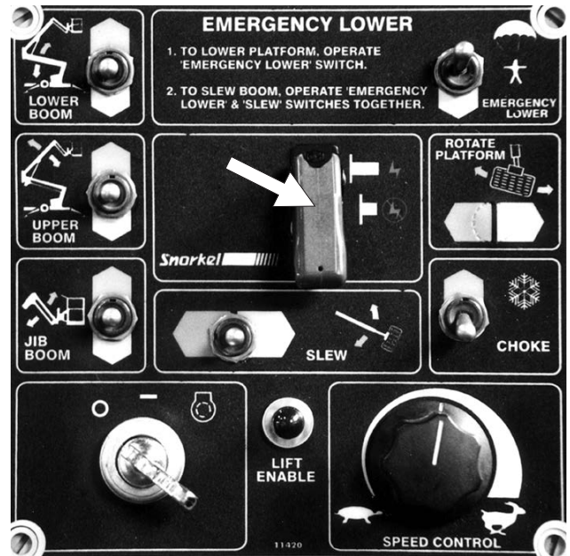
Figure 2.2 - Emergency Stop Switch at Platform Control Box
