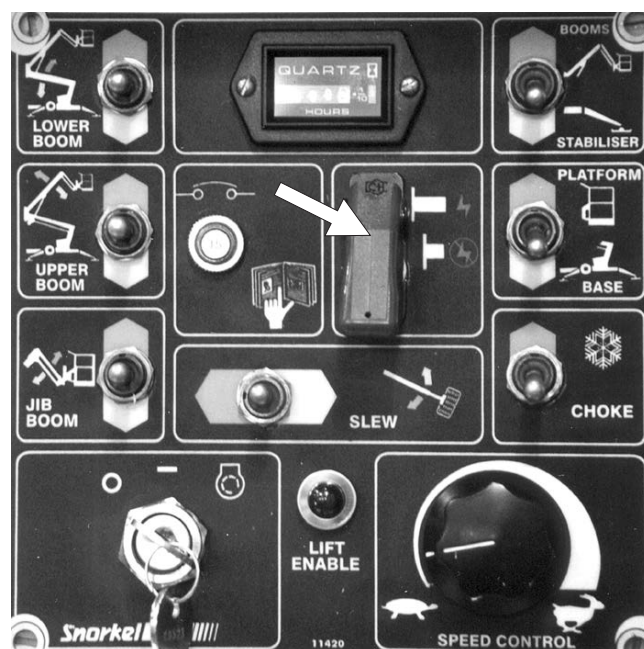
Figure 8.1 - Ground Control Box Emergency Stop Switch Location.
