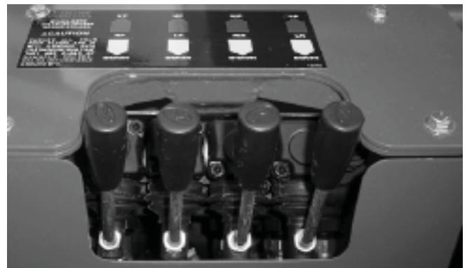
Figure 6.7 - Stabiliser Controls (Manual)
