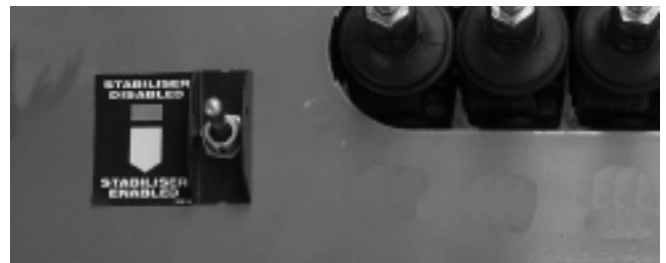
Figure 11.4 - Stabiliser Enable Switch
