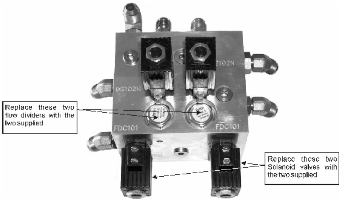
**This picture shows which valves on the manifold need to be changed.**
