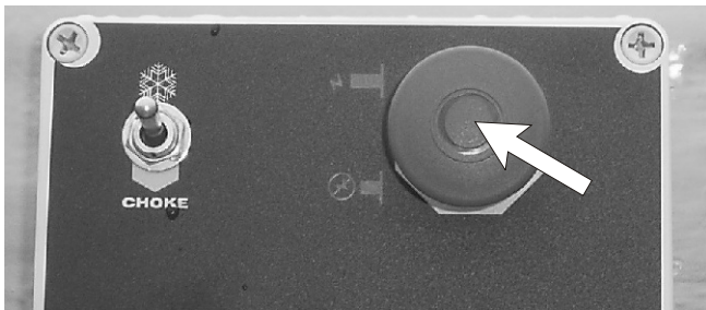
Figure 3.6 - Emergency Stop Switch at Platform Control Box - Non-Insulated Fibreglass Platform
