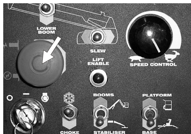
Figure 10.1 - Ground Control Box Emergency Stop Switch Location.
