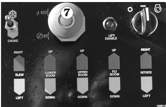
Figure 9.25 - Platform Control Switches - Steel Platform
