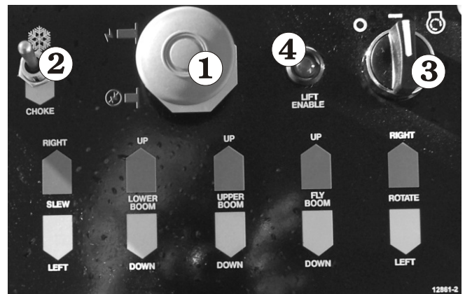
Figure 8.5 - Upper Control Box Controls - Steel Basket
