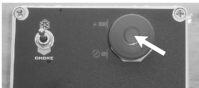
Figure 10.4.3 - Platform Control Box - Non-Insulated Fibreglass Basket, Emergency Stop Switch Location
