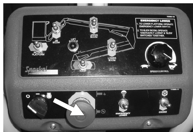
Figure 10.2 - Platform Control Box Emergency Stop Switch Location.
