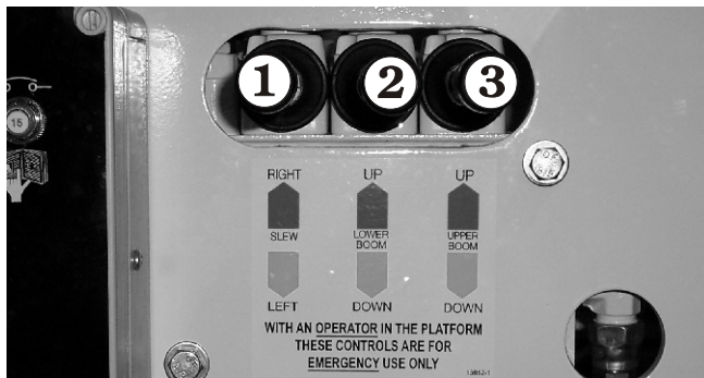
Figure 8.4 - Lower Controls - Movement Control Valve Levers
