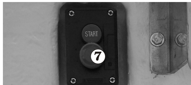
Figure 9.25.2 - Platform Control Switches - Fibreglass Platform
