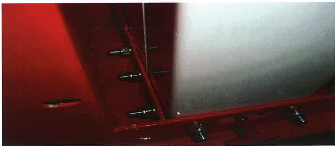
Fig.2 Location of left hand mast bolts. Note the one at the rear does not get changed.
