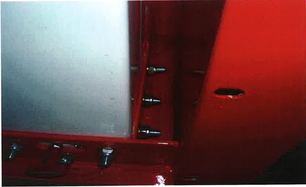
Fig 3. Location of right hand mast bolts. Note the one at the rear does not get changed.
