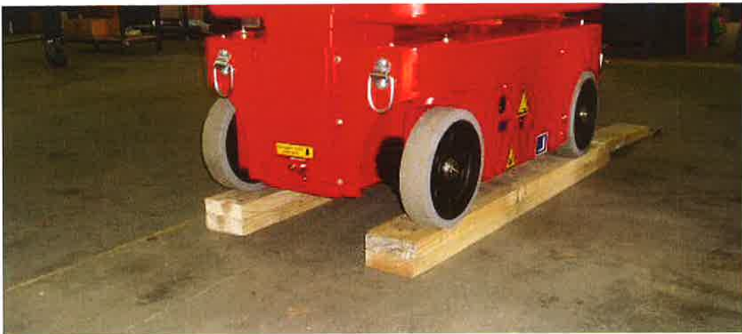
Fig.1 Machine driven onto planks of wood.
