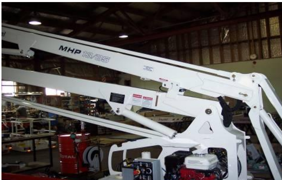
Fig 1 – Booms in position for checking pinkeeper clearance.
