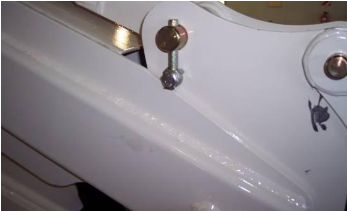
Fig 2 - Pinkeeper touching the edge of the upper boom.
